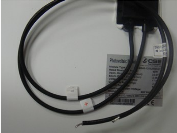
Figure 4: Positive and Negative wires from Solar Panel Array
