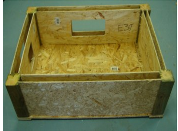
Figure 12: Inner and Outer Walls in place
