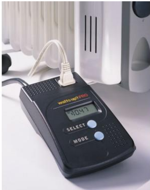
Figure 7: Device plugged into Watts Up Pro Meter
