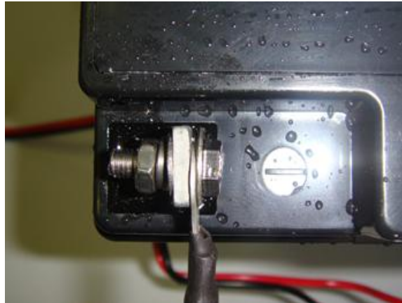
Figure 3: Negative battery terminal (black with – sign)
