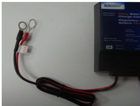
Figure 2: Battery Cords from Charge Controller
