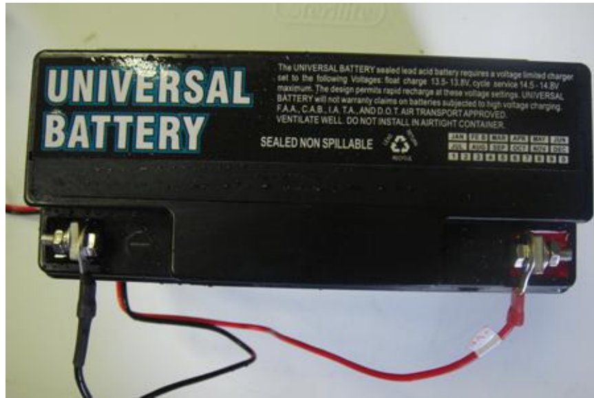
Figure 3: Battery cords connected to positive and negative battery terminals. Notice negative terminal is black with (-) sign, and positive terminal is red with (+) sign.
