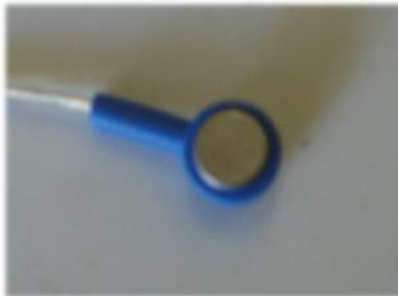
Figure 4: Temperature measuring side of the probe. The other side does not measure temperature
