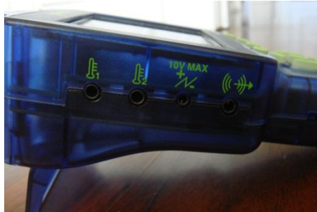
Figure 2: Ports on Side of GLX. Temperature ports are the two leftmost ports.
