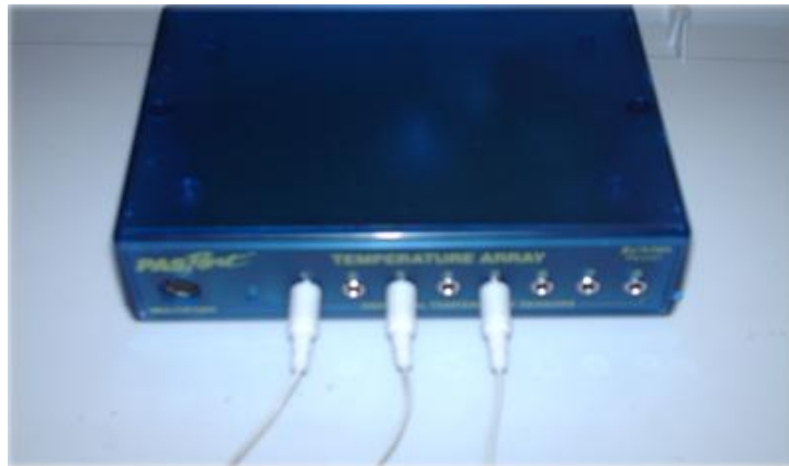
Figure 3: Individual temperature probes connected to input ports on the Temperature Array.
