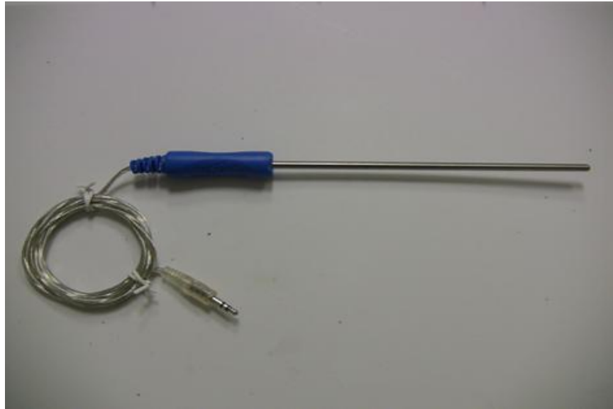
Figure 1: PASPort Stainless Steel Temperature Probe
