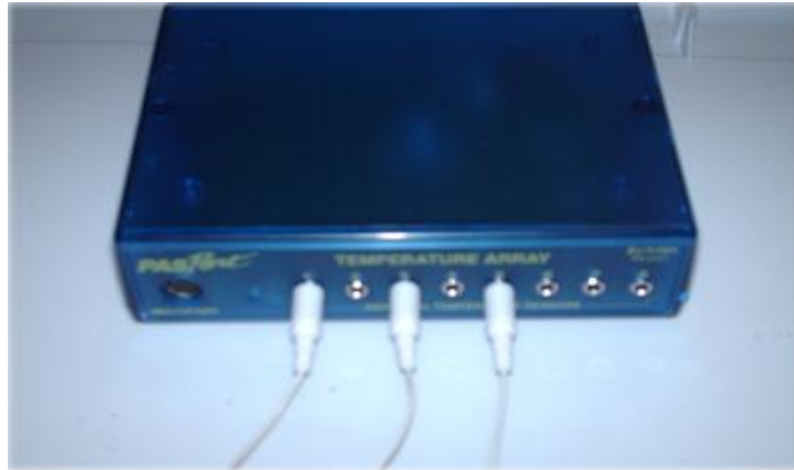
Figure 3: Individual temperature probes connected to input ports on the Temperature Array.
