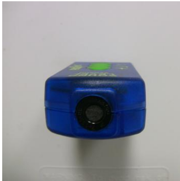
Figure 5: Aperture to be pointed towards source of sound
