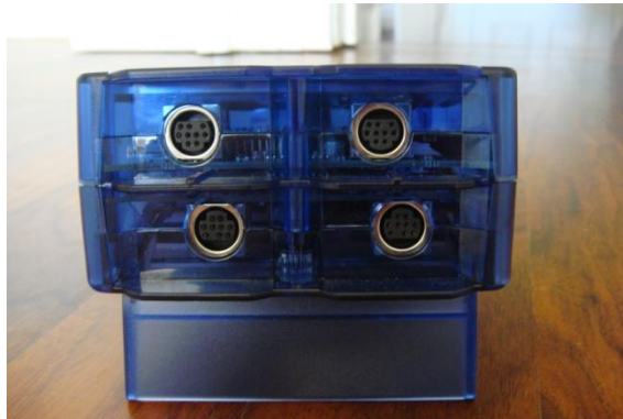
Figure 2: Ports on Top of GLX
