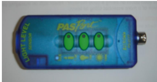
Figure 1: PASPort Light Level Sensor
