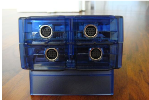
Figure 2: Ports on Top of GLX
