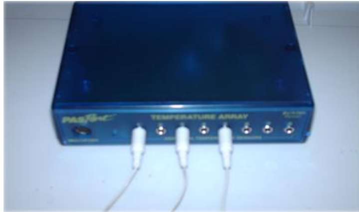
Figure 4: Individual temperature probes connected to input ports on the Temperature Array.
