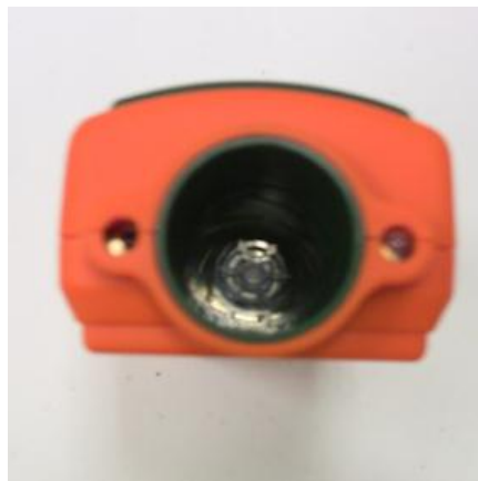
Figure 3: Meter Aperture to be Pointed at Target
