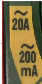
Figure 5: AC Current Dial Settings
