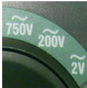
Figure 8: AC Voltage Dial Settings
