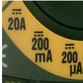
Figure 4: DC Current Dial Settings
