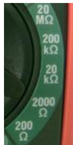
Figure 10: Resistance Dial Settings
